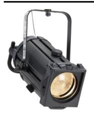
The Acclaim PC is a 300 / 575W / 650W general purpose PC (41/4" diameter lens) for theatre and display lighting which produces a well-defined beam of light, with a crisper edge than a Fresnel that is easily blended with adjacent beams to provide even illumination.
