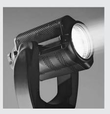
The VARI\*LITE® VL2416<sup>™</sup> Wash luminaire is based on the Emmy<sup>™</sup> Award winning VL5<sup>™</sup> luminaire design. This powerful luminaire uses a 1200W arc lamp and comes standard with a zoomable beam spreading mechanism. An optional collimator/counterweight is available for applications requiring a fixed, collimated beam.
