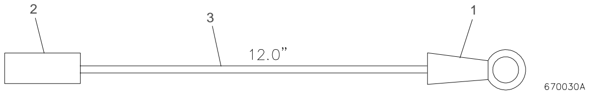
Figure 3-64: Ignitor To Relay Cable Assembly
