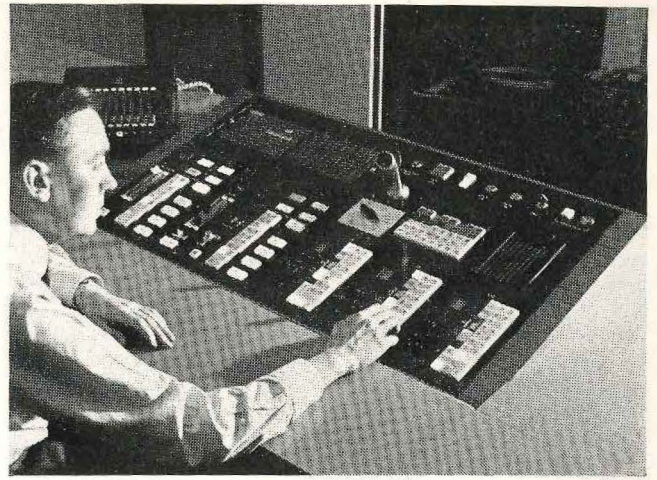
Special Q-File control panel at Studio 8, BBC Television Centre, London
