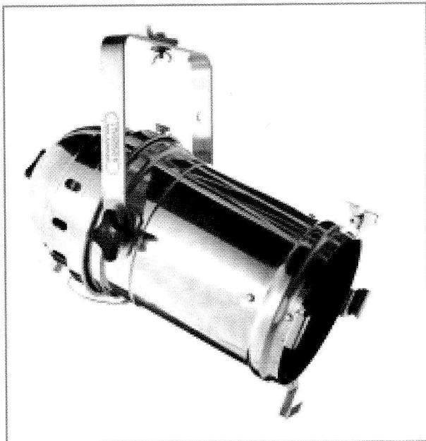
The Brits built PAR cans using spun aluminum for strength and lighter weight. Graham Thomas ran a local metal shop that made electric chicken coop heaters with the process; he would spin PARs for several shops before launching the James Thomas brand.
