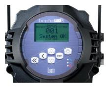
**USER-FRIENDLY CONTROL INTERFACE** With multiple modes and fixture settings including color mixing as 'hue, saturation, brightness' or 'RGB.'
