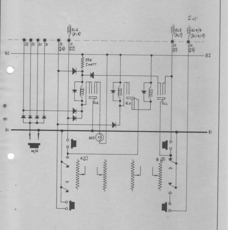
This circuitry is supplementary and is connected in parallel with the manual controls previously described The additional components are mounted within the master desk. The circuit shown opposite is duplicated for the C and D master dimmer levers. The diodes shown are for blocking purposes
