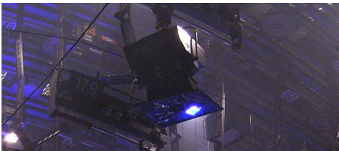
Figure 15. Blue filters with tungsten lighting is not an efficient way to illuminate audiences
