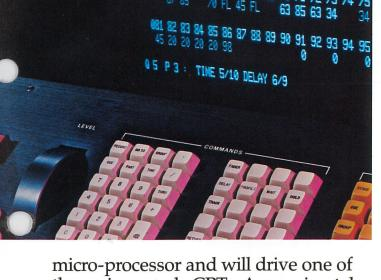
the main console CRTs. Approximately 100 complete cues can be selected from the main memory and automatically loaded into the back-up. The back-up provides a means to select and play back these cues and also to write new ones if required.
