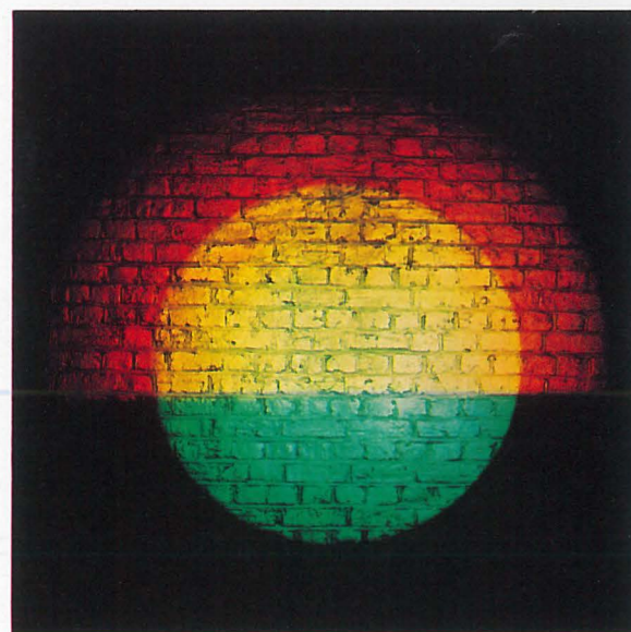
With all the shutters withdrawn to their full extent the 150mm diameter plano-convex lens projects a circular beam which can be hard or soft edged.
