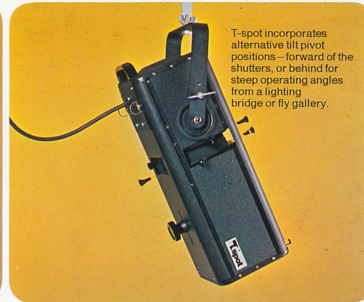
The rear handle assists the setting of the spotlight and there is a large disc and clamp tilt lock on each side. Either clamp gives a positive lock. T-spot is a compact unit only 190mm near square x 560mm long overall, with a textured black finish.
