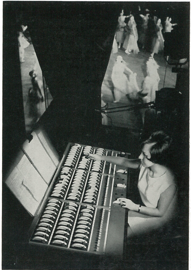
Strand Standard Preset system with 3 presets and control facilities for 60 dimmer channels
