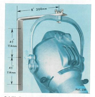
**Ref. 238** Fixed Wall Bracket with two holes for  $\frac{3}{8}$ -in. suspension bolt and wingnut at  $5\frac{1}{2}$ -in. (140mm) and 8-in. (200mm) reach. Weight  $1\frac{3}{4}$  lb. (0·8 kilos).
