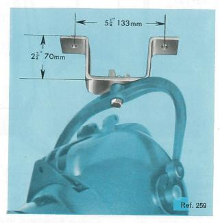
**Ref. 259** Ceiling Fixing Saddle for  $\frac{1}{2}$ -in. or  $\frac{3}{8}$ -in. suspension bolt and wingnut. Weight 1 lb. (0.45 kilos).
