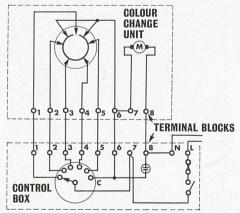
Ref. 600 7-core control cable, with an external diameter of  $\frac{3}{8}$ -in. (10mm), is recommended for interconnection. If continuous rotation only is required the AC supply should be connected to terminals 7 and 8 at the colour change unit.
