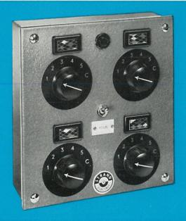
Five of the positions of each control switch are numbered and each selects the corresponding aperture at the colour change wheel which rotates until the chosen aperture is brought to rest before the lens of the spotlight. A neon pilot above each switch remains alight while the motor is in operation. The sixth position of the switch, marked C, provides continuous rotation.
