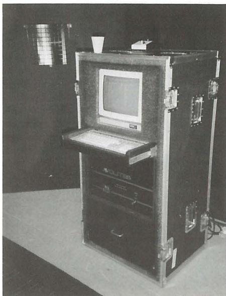
Avolites new computerised chain hoist controller for complex road show rigs.
