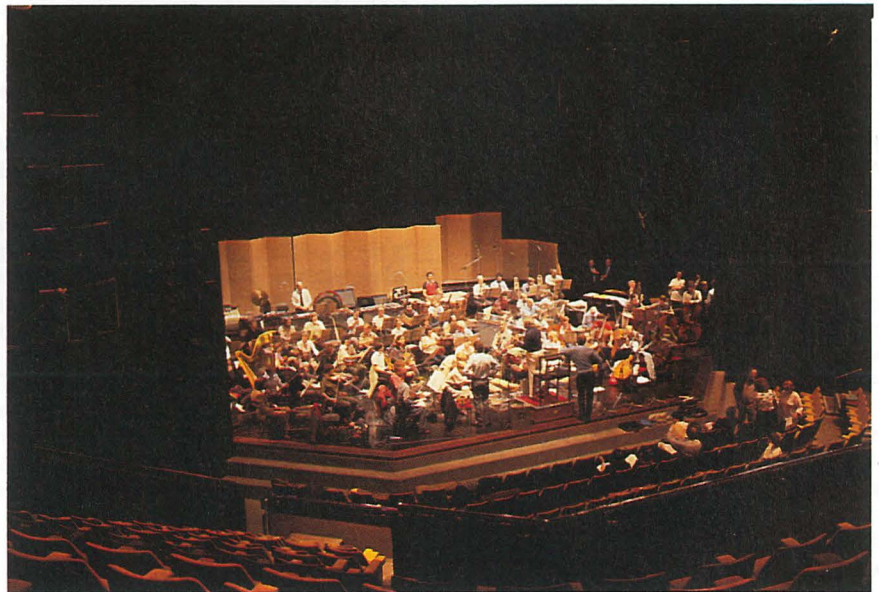
The tall lightweight screens behind and around the orchestra provide diffuse mid/high-frequency reflection.
