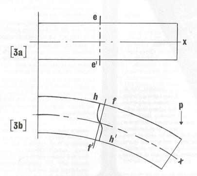
The diagrams which follow demonstrate that a designer has to arrange the materials of the core (web of a beam) to give the best configuration to absorb all the stress created when the structure is loaded, if the quantity and type of material used is to be kept to a minimum consistent with maximum performance.
