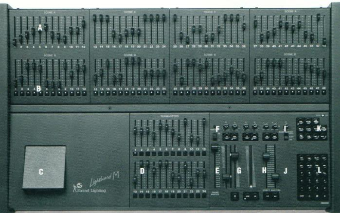
**J** Special Effect **Playbacks** Two separate special effect sequences can be played back with proportional masters, START/STOP buttons and step time override
