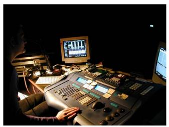
Finally, you can make modifications to channels through ranges of cues. For example: [1] [UPDATE] [CUE] [1] [THRU] [10] [@] [50] [\*] will set channel 1 at 50% through these cues ("put the wing workers on at 50% through the entire show"). Note that you'll have to vary how you type the level depending on whether you're in single digit, double digit or command line entry mode ([SETUP] > Channel Control Mode).
